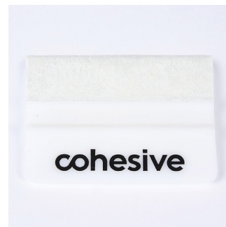
CODE: VXAWT COHESIVE APPLICATOR - FELT EDGE FIRM - Plastic side used to affixed Decals covered with application tape. Soft felt side is used for application of large areas of self-adhesive film.
